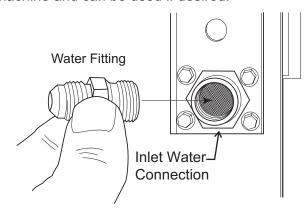
Water cooled models have the same inlet fitting plus an additional 3/8" FPT condenser inlet water connection.
